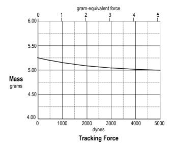
Again, the graph shows us the counter-intuitive effect of the mass decreasing with increasing tracking force, even though the dependence is small, at best. In our example, increasing the tracking force from 1000 to 5000 dynes, an increase of 500% or a factor of 5, results in a reduction of mass of only 3%, a negligible change, at the worst.
